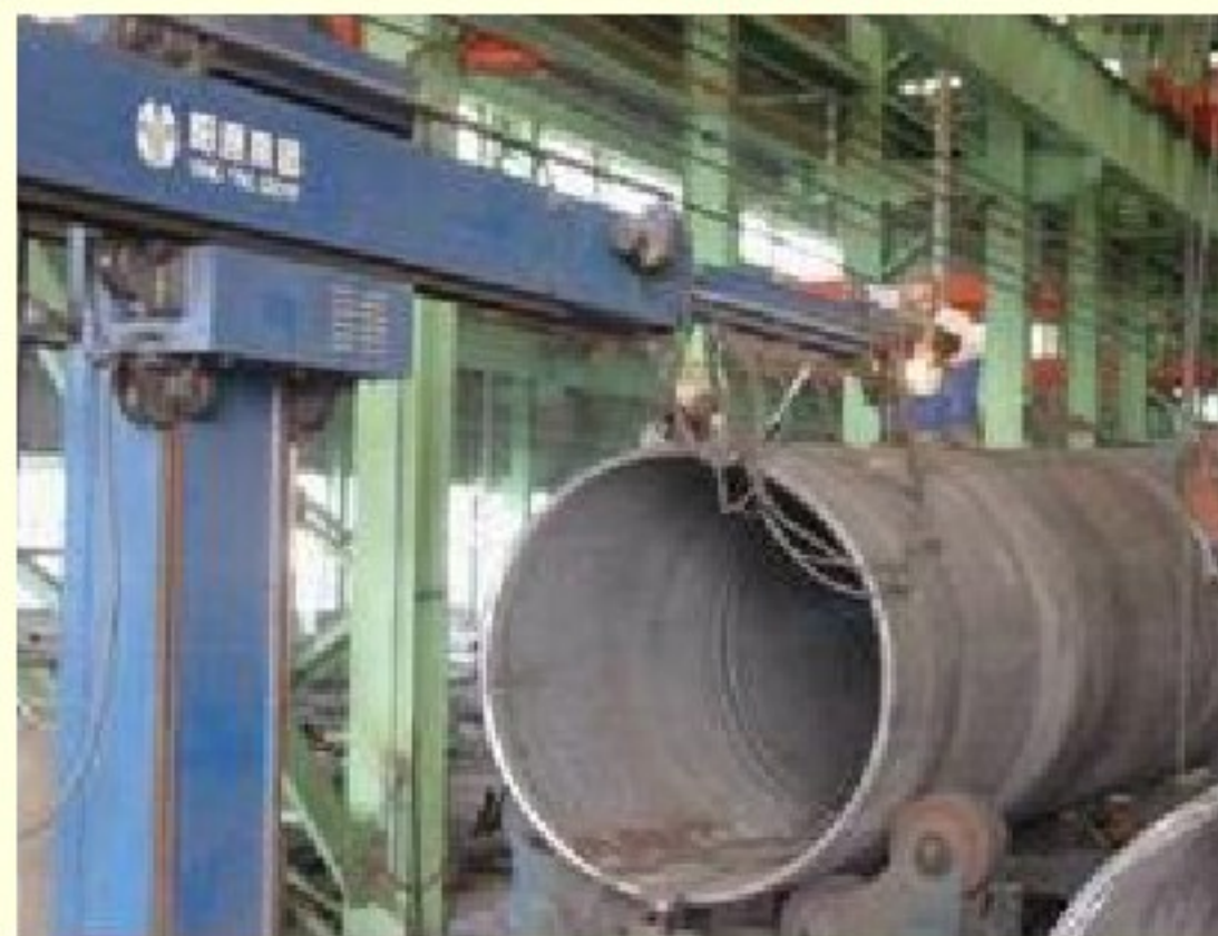
SAW 焊接环焊缝
